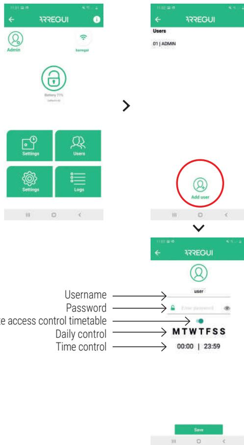
Once you’ve finished configuring the options, press the “SAVE” button. The knob will light up in green to confirm that the settings have been saved correctly.
